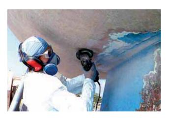
**3** Smoothing with an elliptical planing machine (outfitted with heat-resistant blades) and subsequently disc sanding with rotary or orbital disc sanders.
