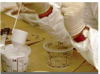
The choice of the undercoat depends on the substrate material, the desired result and on the application procedure. Air pressure, paint viscosity, number and thickness of coats, distance of the spray gun from the surface and spray technique depend on the experience and ability of the operator.
