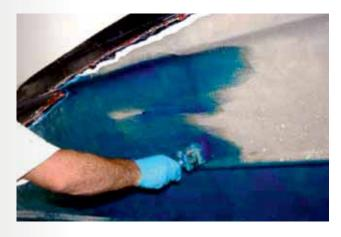
7 After a drying interval of 16 hours minimum and 48 hours maximum (at 20° C), smooth all imperfections with the filler EPOMAST EVO, which has a low specific weight and therefore doesn't affect the weight of the boat significantly.
