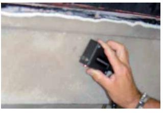
The hull can be considered dried out when the measured humidity content is below 10%.
